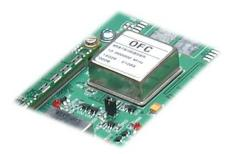
The Ovenized Crystal Oscillator (OCXO) upgrade improves holdover accuracy. By keeping the crystal oscillator at a fixed temperature, if the GPS signal is lost, thereby placing the server in holdover, the OCXO reduces clock the drift.
