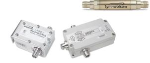
Antenna cable accessories enable versatile solutions that are simple to achieve. Inline GPS amplifiers are an easy way to extend cable runs from 150 feet (45 meters) to 300 feet (90 meters). Lightning arrestors provide valuable electrical shock protection to the SyncServer. Antenna cable splitters leverage a single antenna and cable between two GPS equipped time servers.
